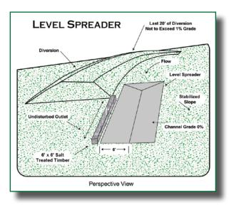
The level spreader will release directed flow from a drainage structure, such as a lead-off ditch, to a zero grade and release it into the undisturbed forest area as sheet flow.
