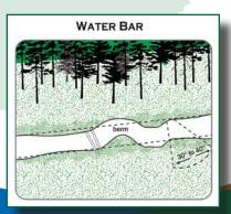
Upon completion of skidding activity, water bars should be installed immediately in areas subject to erosion.
