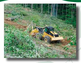
Shovel – Shovel logging is limited to clear cutting when it is necessary to pick up and swing the timber toward the road. Shovels can work in adverse weather, in wet areas and on steep slopes.
